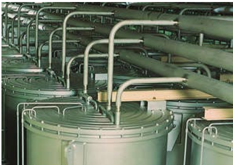
Photo: Cascade at Rokkasho Uranium Enrichment Plant
