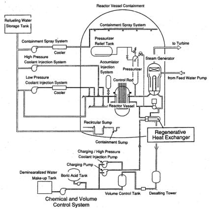
links primary coolant system and chemical and volume control system.
