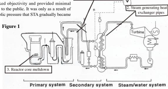
1. Sodium leakage accident
