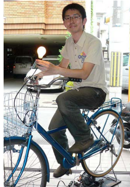
The pedal-power bicycle generator is lighting the lamp. Mr. Yamami is involved in the development of pedal power generators.
